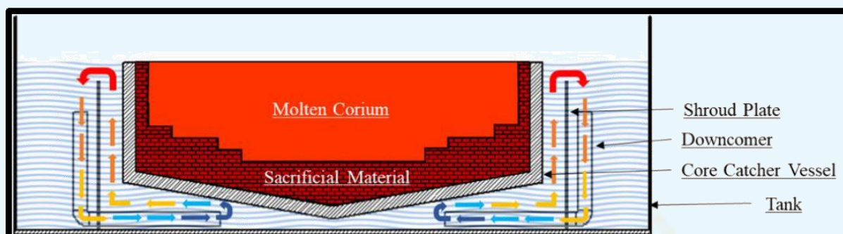
Schematic showing proposed core catcher vessel model
